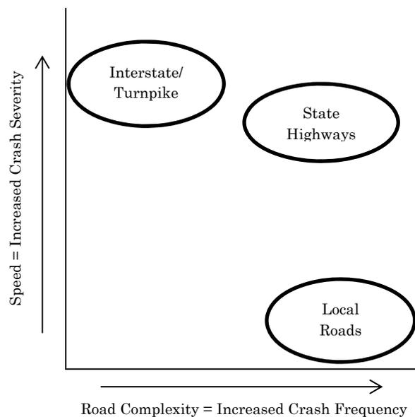
Figure 1. Road Speed vs. Complexity<sup>52</sup>
